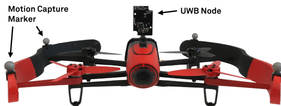
Fig. 2. Modified Parrot Bebop 1 st generation used in this work.
