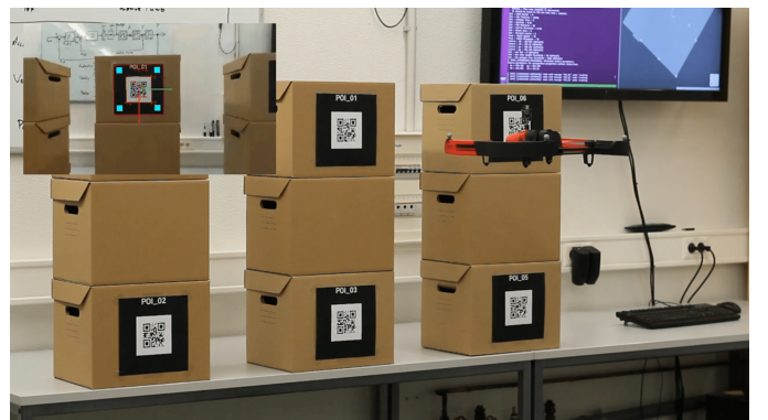
Fig. 13. Still of the interactive application video [19]. The UAV is searching for a QR-code labeled box in the warehouse-mockup.
