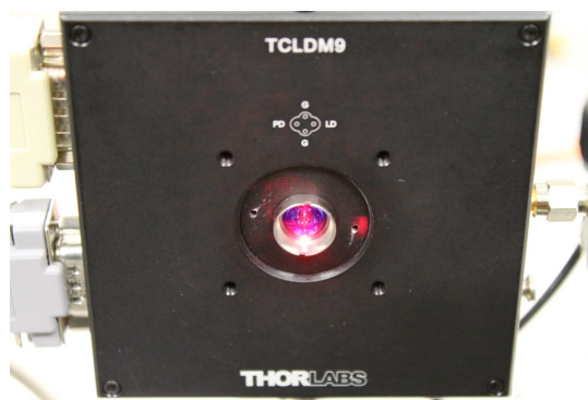
(d) A QPHOTONIC® QSDM-680-9 SUPER-LUMINESCENT DIODE in a THORLABS® TCLDM9 cooled laser mount.
