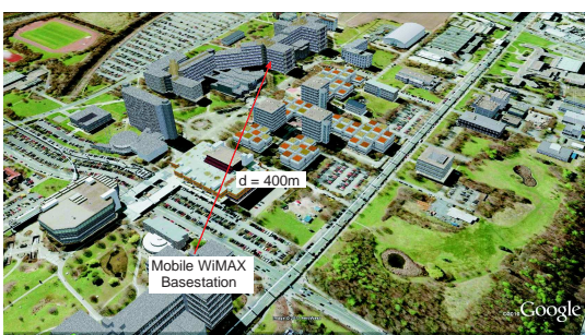
Fig. 7. Mobile WiMAX Link for Validation Measurement, (c) 2011 Google
