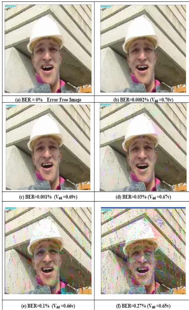
Fig. 7 Snap shot of CIF-sized "FOREMAN" video image (29 th frame where an I-frame comes every 30 th .) Encoding Configuration : IPPPP, QP=28, Reference Frame#=2, I frame Period=30
